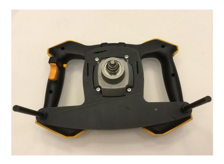
Attach the rods to the plate first.
